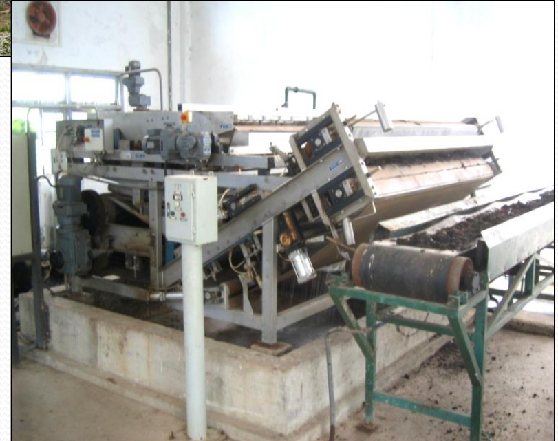
Belt Press Machine Capacity -800 kg Sludge Cake /hr
